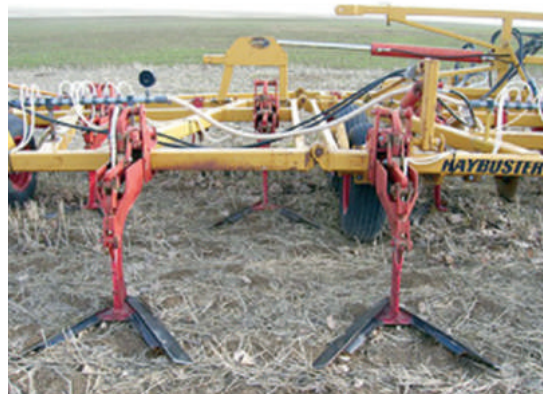
An undercutter with V-shaped blades used for primary spring tillage with fertilizer injection during the fallow year. Photo by Harry Schafer, Washington Association of Wheat Growers
