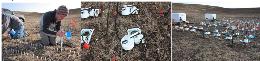
Figure 2.3. Injection of N fertilizer on chamber study microplots, automated chambers, and chamber, environmental sensor array at the CAF
