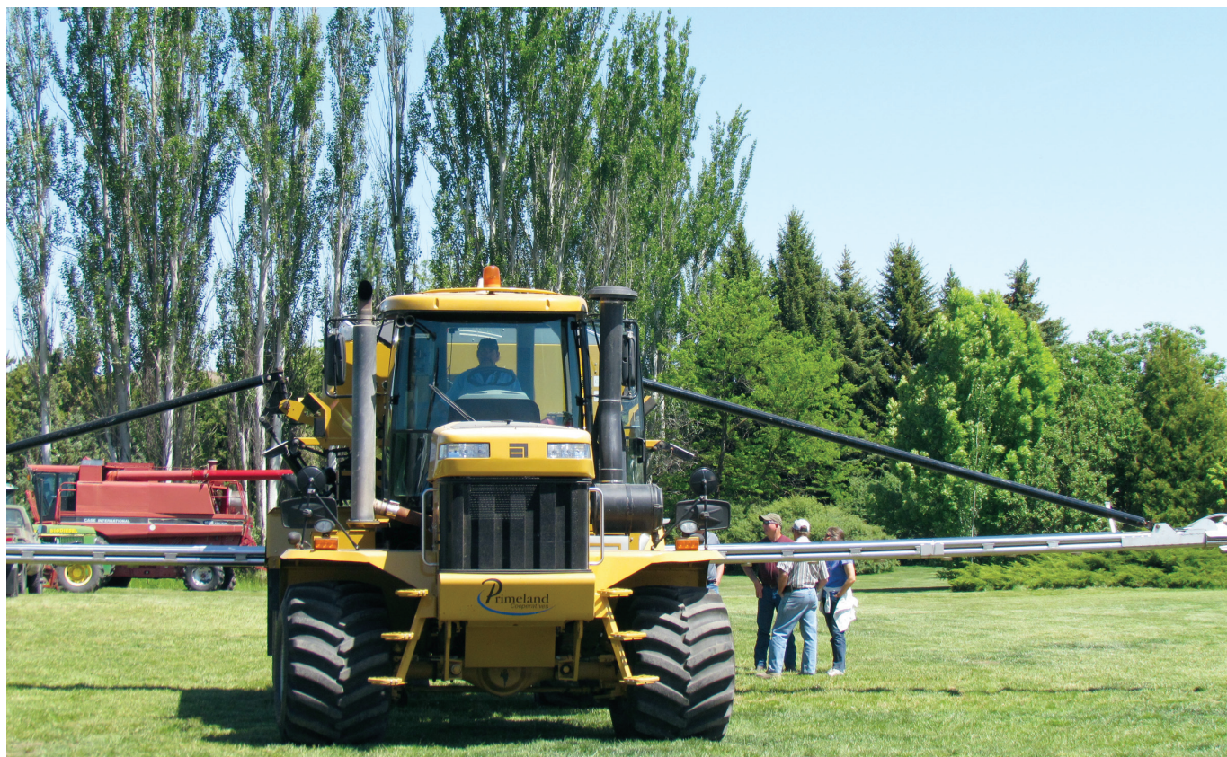
Figure 1. CHS Primeland displays a dry fertilizer applicator equipped with precision technologies at a June field day in Moscow, ID. Photo by Leigh Bernacchi.
